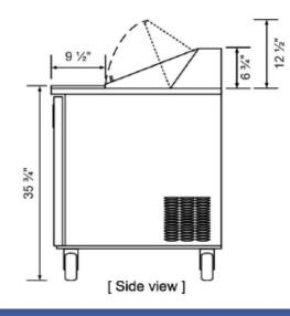
Crated Holding Width Depth Height Weight Voltage Refrigerant Cubic ft Нр Amps Temp 60.4" 33.0" 42.8" 362 LBS 115V/60Hz 3/8 6.0 R134A 16 32°F to 45°F Beltsville, MD 20705 USA **6890 Distribution Drive**
